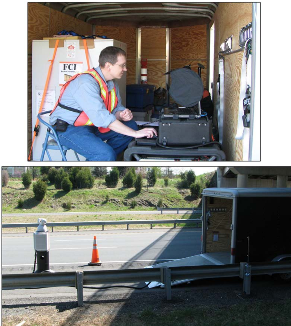
FIGURE 20 Instrument setup and operation for impact damage measurements.
