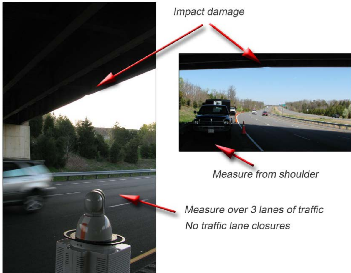
FIGURE 17 Measurement of impact damage on Virginia Bridge 4021.
