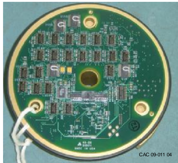
FIGURE 4. Single Board Computer
