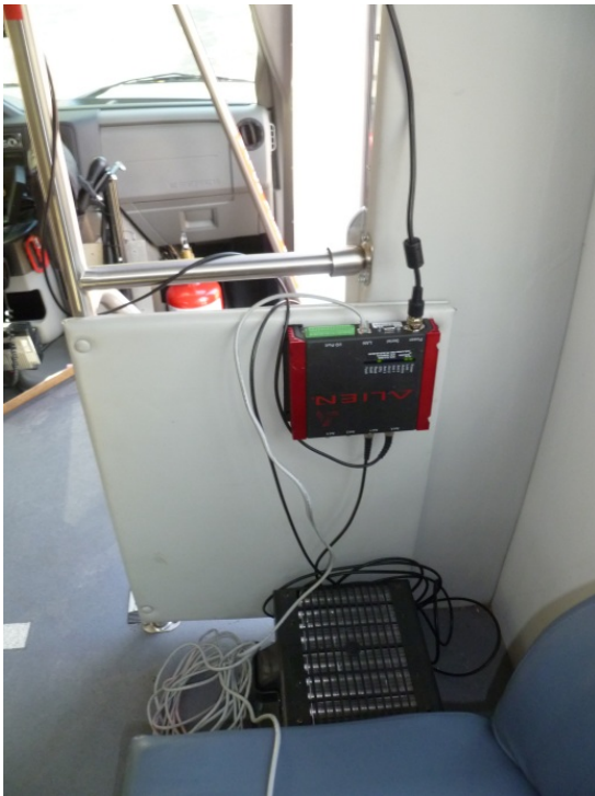
FIGURE 3.3 RFID reader mounted in paratransit bus
