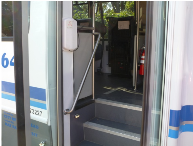
FIGURE 3.4 Front RFID antenna in paratransit bus
