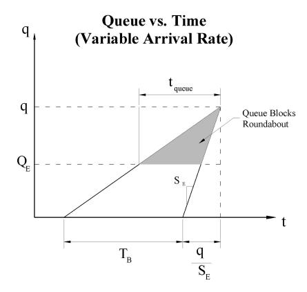
Once the probabilities and durations of each queue length are known, one can estimate the average duration of queue blocking for each blocking event by determining the probability of a queue of length q and multiplying it by its duration. Short queues have a high probability but low duration, and long queues have a low probability but high duration. This is shown as follows:
