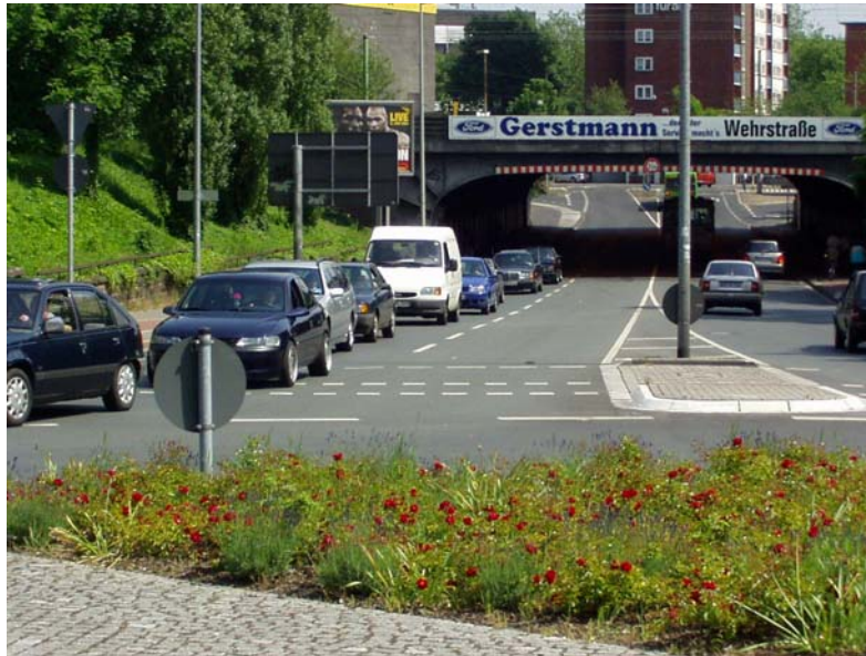
Fig. 9: Typical driver behavior at a compact two-lane roundabout: unused left lane on a two-lane entry
