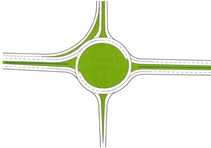
fig. 10: Large Roundabout with Addition of Inner Lanes (RAIL) at the entries and one bypass within a 4-lane arterial.
