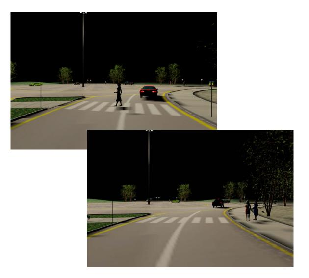
For the roundabout with approach lighting we used 8-10 meter poles with 250 watt high pressure sodium full cutoff cobra head luminaries.
