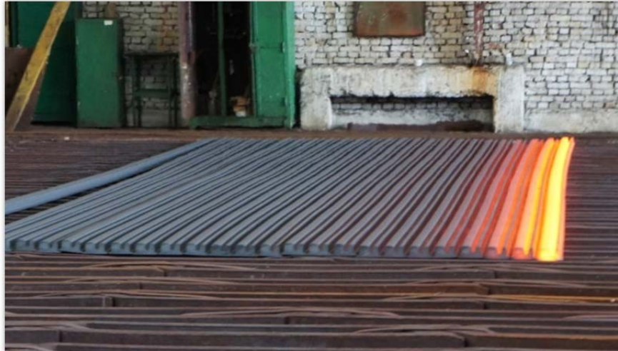
FIGURE 3 Block rail cooling after rolling.
