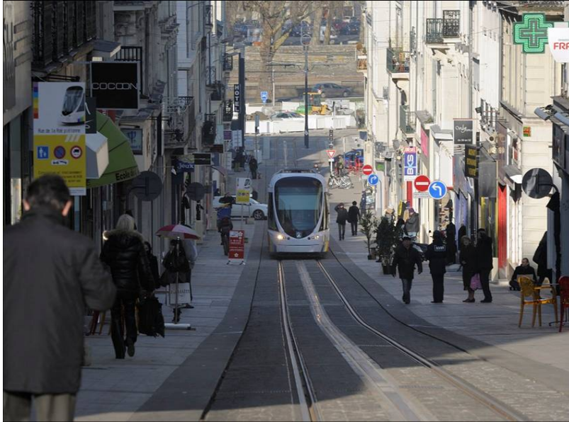
FIGURE 7 Alternate running on single tracks, Roë Street, Angers.
