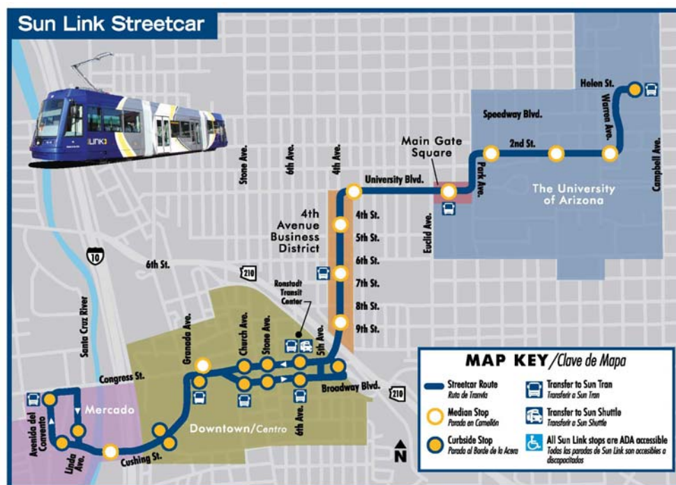
FIGURE 5 Tucson's Sun Link system was designed with a stop across the street from the downtown bus transit center. This, along with other bus connection points, is illustrated on the Sun Link system map.
