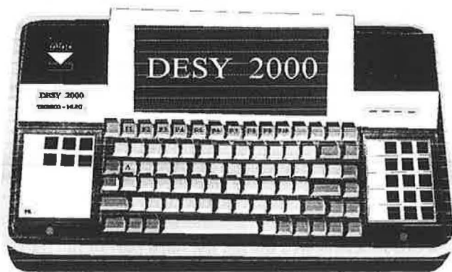
FIGURE 1 Computer-assisted recording system DESY used for damage survey (with its two specialized-function keypads).
