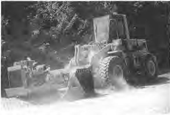
FIGURE 3 F.A.H.R. single-rotor crusher retrofitted to a front-end loader.
