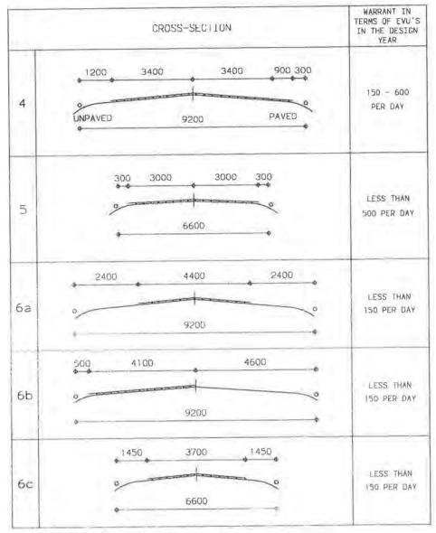
FIGURE 1 Cross sections for low-volume roads.
