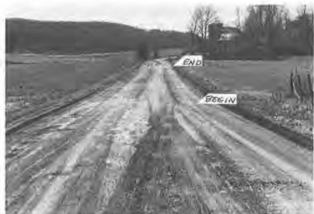
FIGURE 5 Overview of tire chip section, April 3, 1991. Note surface moisture on adjacent untreated sections.
