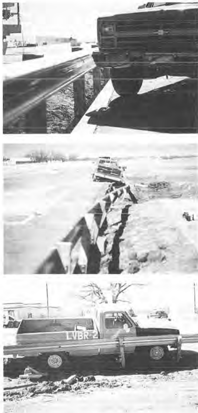
FIGURE 7 Impact location, vehicle trajectory, and vehicle damage, Test LVBR-2.
