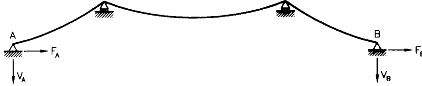
FIGURE 2 Definition of forces at ends of cable.
