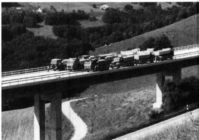
FIGURE 1 Load test of Daillard bridge in French-speaking Switzerland.
