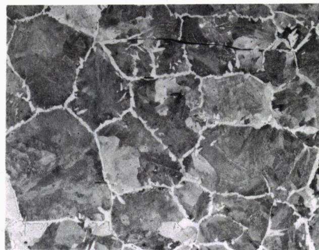
FIGURE 12 Flange plate microstructure of Core 17 (77 \times ).
