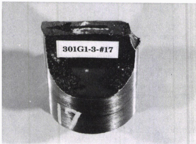
FIGURE 7 Core 17 showing transverse weld metal crack extending into flange; Cores 23 and 25 are similar. Arrow on web indicates west direction.
