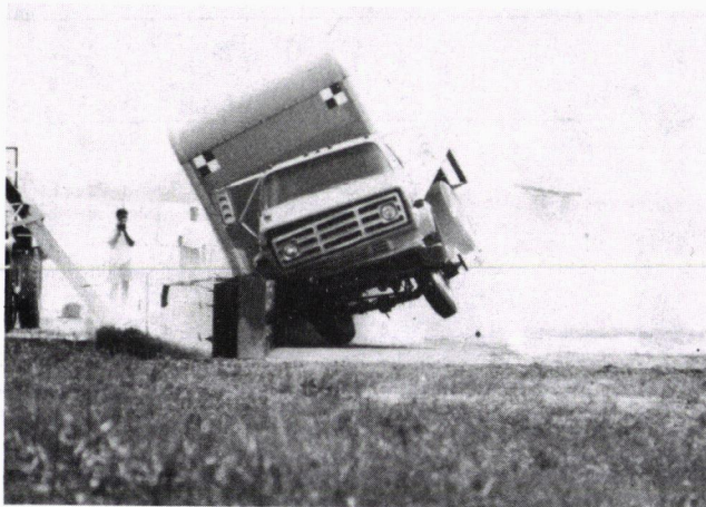
FIGURE 1 Crash-test sequence for 8172-kg (18,000-lb) truck traveling at 80.5 km/hr (50 mph), hitting railing at 15-degree angle to longitudinal railing axis.
