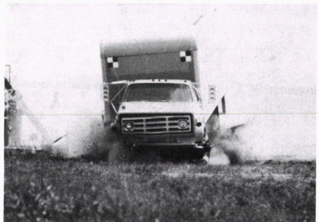
FIGURE 1 Crash-test sequence for 8172-kg (18,000-lb) truck traveling at 80.5 km/hr (50 mph), hitting railing at 15-degree angle to longitudinal railing axis.
