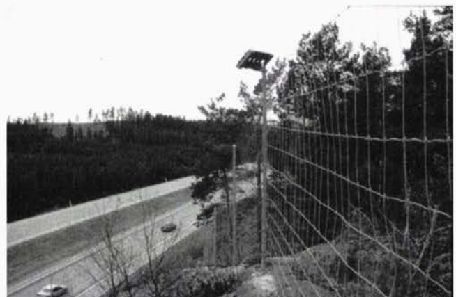
FIGURE 4 Steel plates for monitoring atmospheric corrosion.
