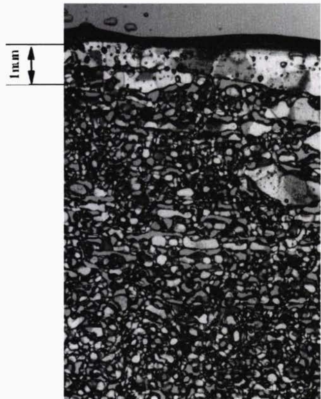
FIGURE 8 Thin layer of compacted snow from extremely slippery road observed through a polarizing microscope.
