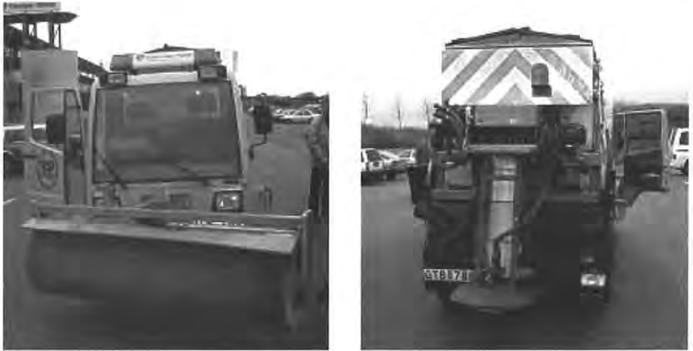
FIGURE 2 Mercedes Benz UX 100 equipped with a front-mounted sweeper for snow clearance and a spinner for spreading salt, brine, or grit.
