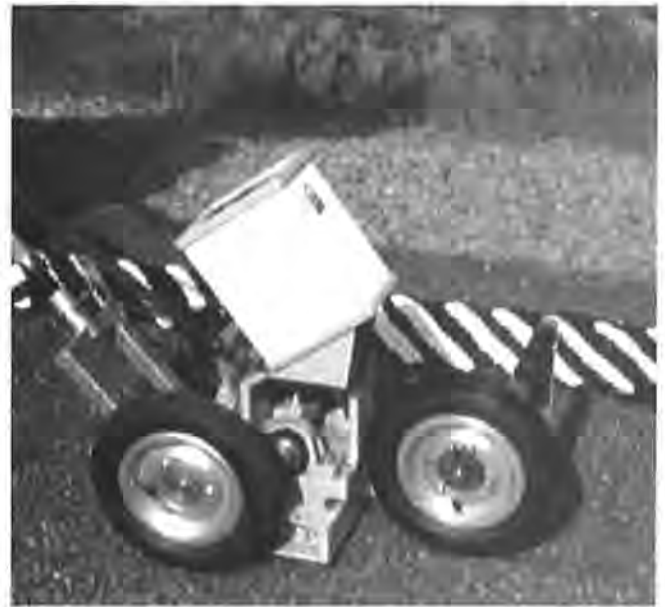
FIGURE 5 Portable friction tester, constructed at the Swedish National Road and Transport Research Institute for measuring the friction over short distances.
