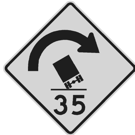
Figure 13. Truck rollover warning sign typically used at curves on interchange ramps.
