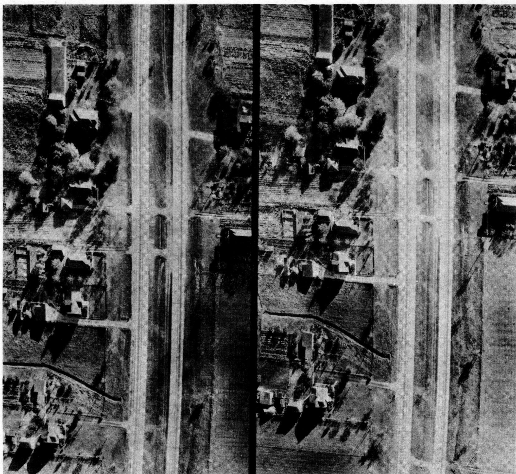
Figure 1. Illustration of Continuous Strip Aerial Photography
