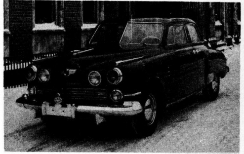
Figure 2. Polaroid and City Headlamps Installed
