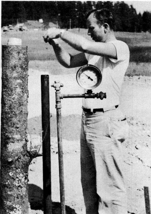
Figure 12. Checking water rise against pressure piezometric gauge. Vacuum of \pm 1\frac{1}{2} inches initially applied. Gauge reads in pounds per square inch plus and inches of mercury minus.
