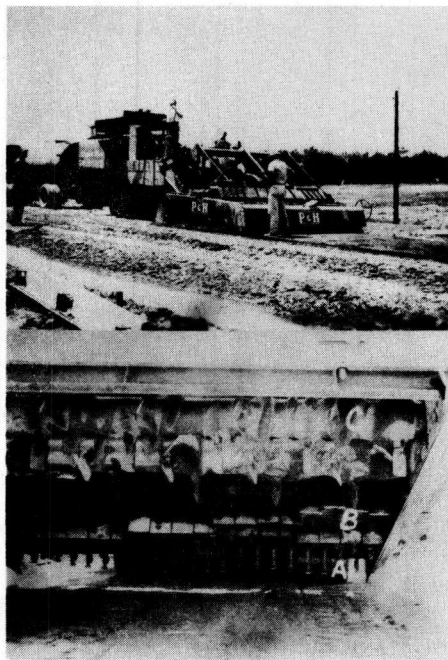
Figure 12. Equipment used in processing soil-cement subbase material. At top is rear view of the single-pass processing unit; at bottom, mixer box elevated to show: (A) cutting rotor; (B) shaping blades; and (C) mixing blades.
