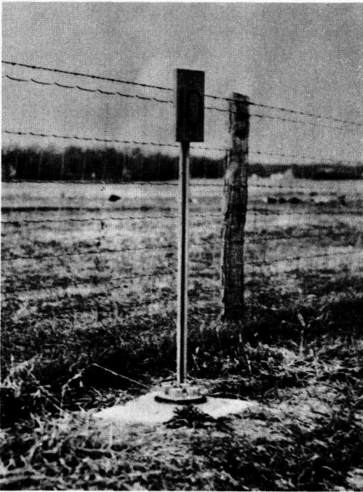
Figure 6. Completed frost-proof bench mark.
