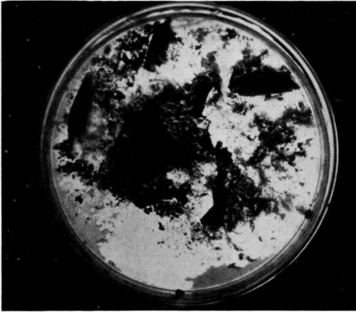
Dark Portion - Remains of Oil Film. The Results of Oil No. 1 on Inoculated Salt Media -Color is gray to Biege Light gray is fatty acid residue.
