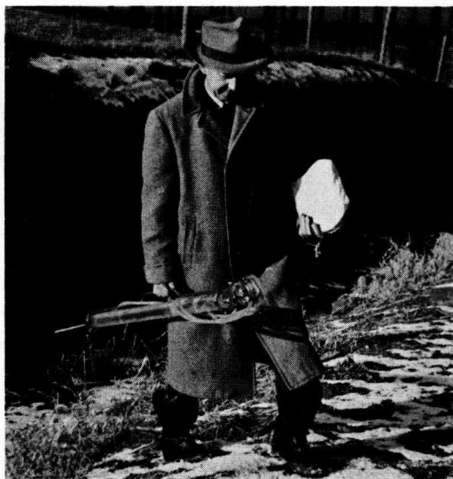
Figure 4. Apparatus assembled for carrying. The balloon holder and loose hose fasten onto the graduated cylinder support, and (right) the folding template fits into the sample bag for carrying.
