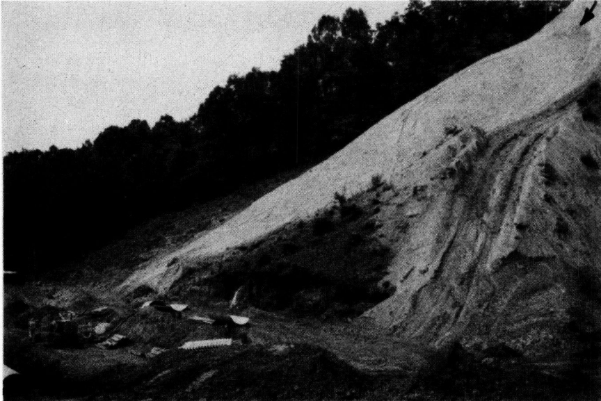
Figure 9. Beginning of slide. Arrow points at trace of failure surface shown clearly on picture.
