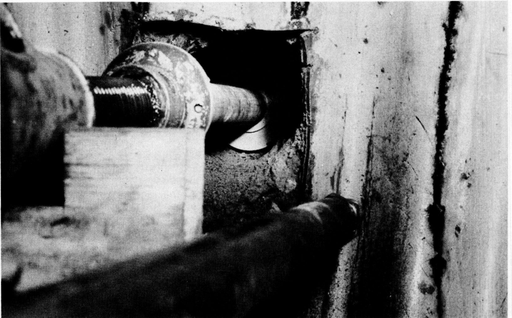
Figure 23. The sampling device forced into the side supporting material to obtain the second soil sample from this opening.
