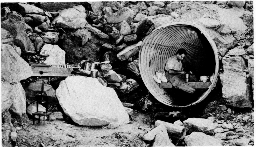
Figure 27. Trimming ends of soil sample trapped inside the main chamber of the sampling device. Shown on the left side of picture: scales for density determination of samples, soil core extracting apparatus, and moisture cans by means of which samples were taken to the N.C. State Highway Laboratories to be analyzed.
