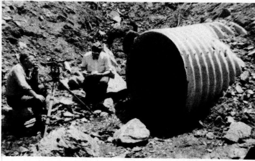
Figure 28. Obtaining profile of culvert flow line. Instrument man was able to communicate with rodman through a two-way telephone line.
