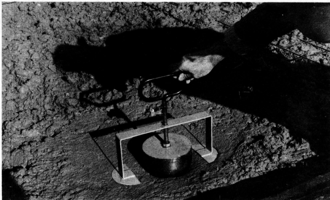
Figure 2. Kelly ball penetration test as used in the field.
