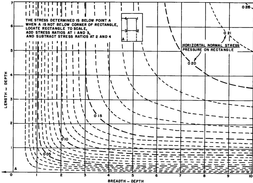
Figure C. Graph of horizontal normal stress under corner of rectangle loaded with unit pressure.
