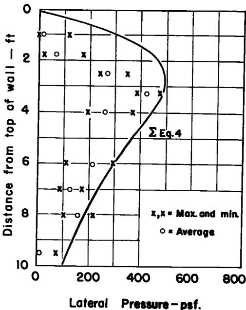
Figure 22. Lateral pressures caused by surcharge only, backfill number four. Surcharge number two, 1,448 psf at 2 feet clear distance from wall.
