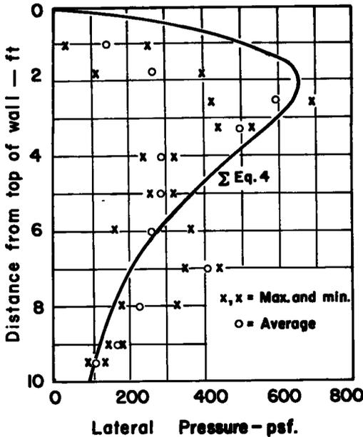
Figure 25. Lateral pressures caused by surcharge only, backfill number four. Surcharge number three, 1,448 psf at 3 feet clear distance from wall.
