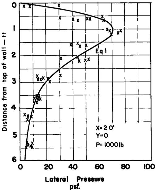
Figure 4. Lateral pressure due to concentrated load - 1934.
