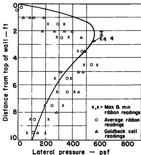
Figure 11. Lateral pressure due to area load - 1941.
