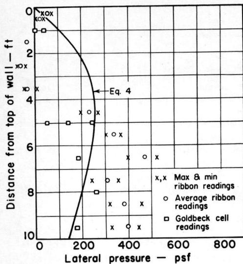
Figure 13. Lateral pressure due to area load - 1941. Load 6 feet from wall.
