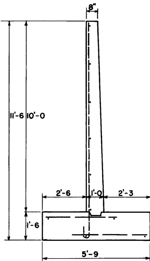
Figure 8. Cross section of experimental wall - 1940.
