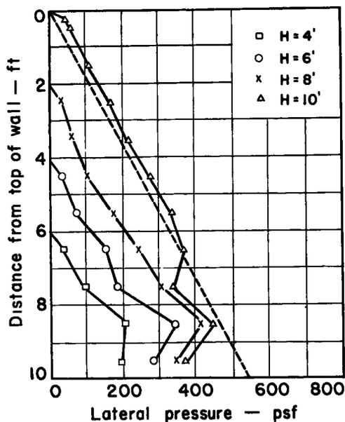
Figure 10. Lateral pressure, backfill only - 1940.
