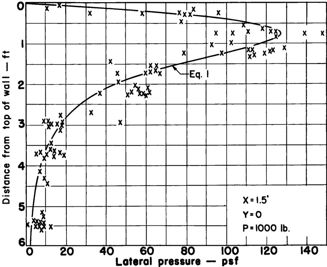
Figure 3. Lateral pressure due to concentrated load - 1934.
