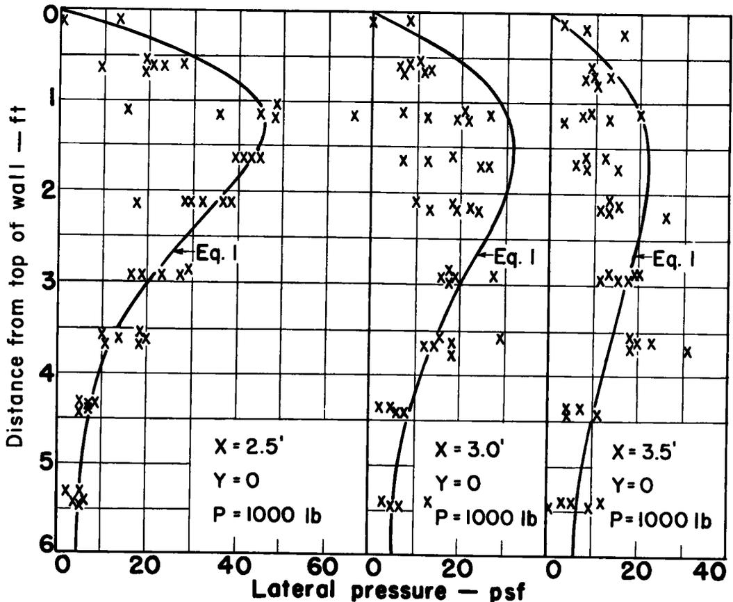
Figure 5. Lateral pressure due to concentrated load - 1934.
