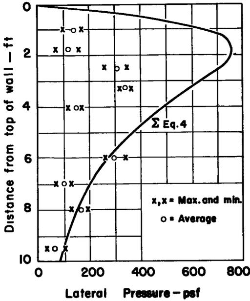
Figure 23. Lateral pressures caused by surcharge only, backfill number three. Surcharge number two, 1,448 psf at 3 feet clear distance from wall.
