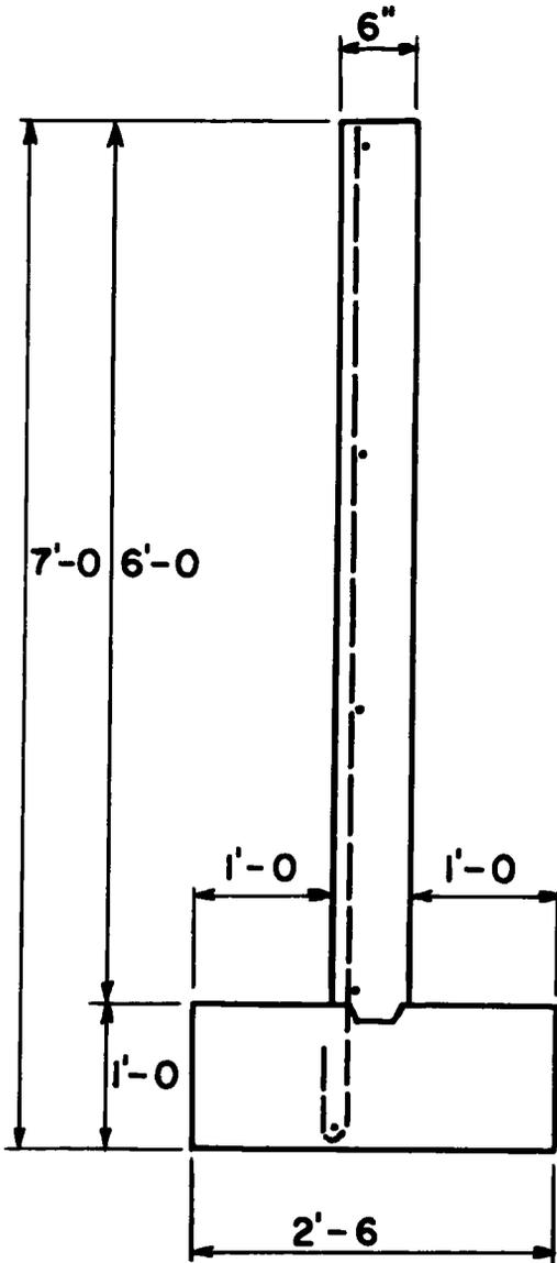
Figure 2. Cross section of experimental wall - 1932.
