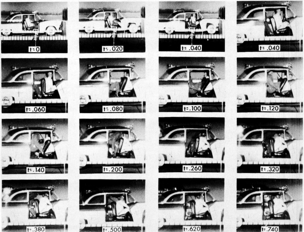
Figure 18. Crash 39 - Test dummy kinematics during impact.
