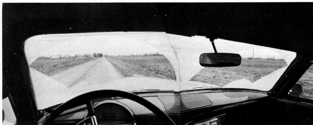
Figure 5. Standard windshield-wiper pattern on a 1954 Ford sedan, using extra-length blades (12 in. instead of 11 in.) on the conventional equipment supplied with the automobile, where the wipers point to the center when parked flush with bottom of windshield. The three pictures show the outside areas seen through the pattern as in actual operation by drivers of various heights from very short to very tall. Note the marked improvement from (a)-(b), and in (a) the vehicle on the road ahead largely concealed by the wheel.
