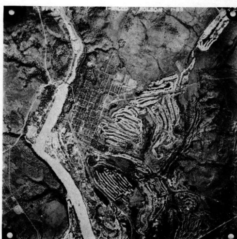
Figure 1. Contact prints at some of the scales being used for freeway planning and design. Scales of original photographs: upper left, 1 in. = 250 ft; lower left, 1 in. = 400 ft; upper right, 1 in. = 1000 ft; lower right, 1 in. = 2000 ft.
