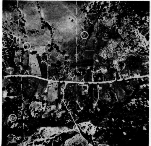
Figure 4. The primary ground control survey for an 8-mi design mapping project is shown in the upper diagram. The overlapping aerial photographs below illustrate the photo control points established for one of the stereoscopic models.
