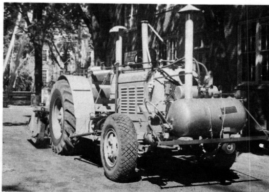
Figure 5. Steam boiler attachment.
