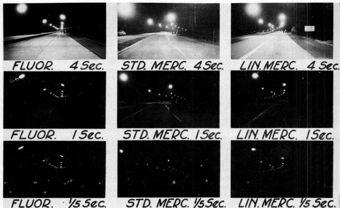
Figure 1. Luminaire located about 50 feet in front of camera. (Courtesy of "Illuminating Engineering")
