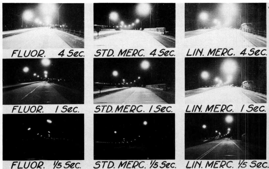
Figure 2. Luminaire located about 50 feet behind the camera. (Courtesy of "Illuminating Engineering")
