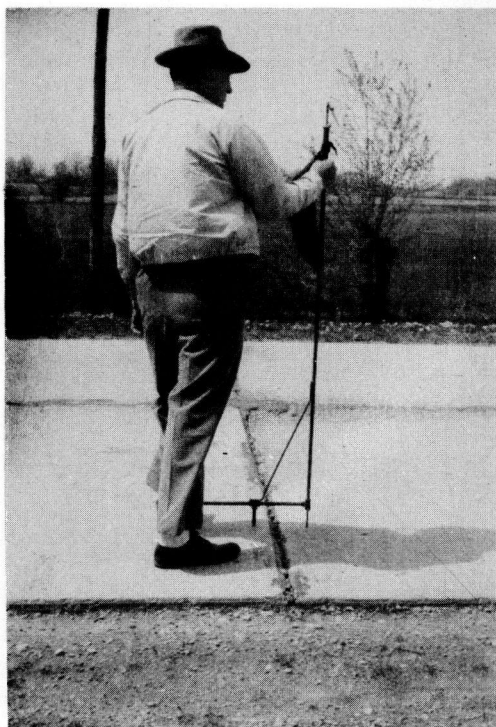
Figure 12. Instrument and method used to determine the amount of faulting at all cracks and joints.
