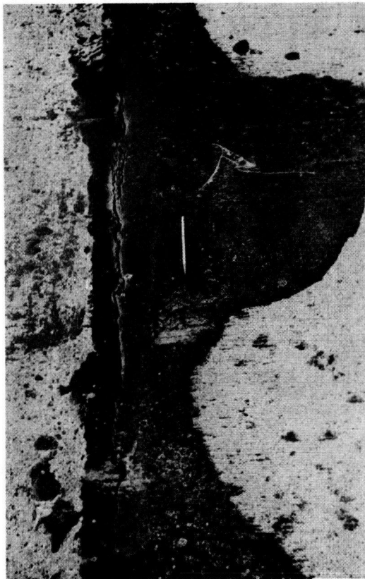
FIGURE 18. FAILURE MAINLY IN COHESION ; TYPICAL OF BRAND A FAILURES AT 2 1/2 YEARS.
