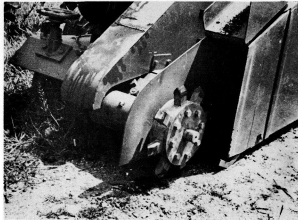
FIGURE 4. CUTTING HEAD OF CONTRACTOR'S JOINT - CLEANING MACHINE.
