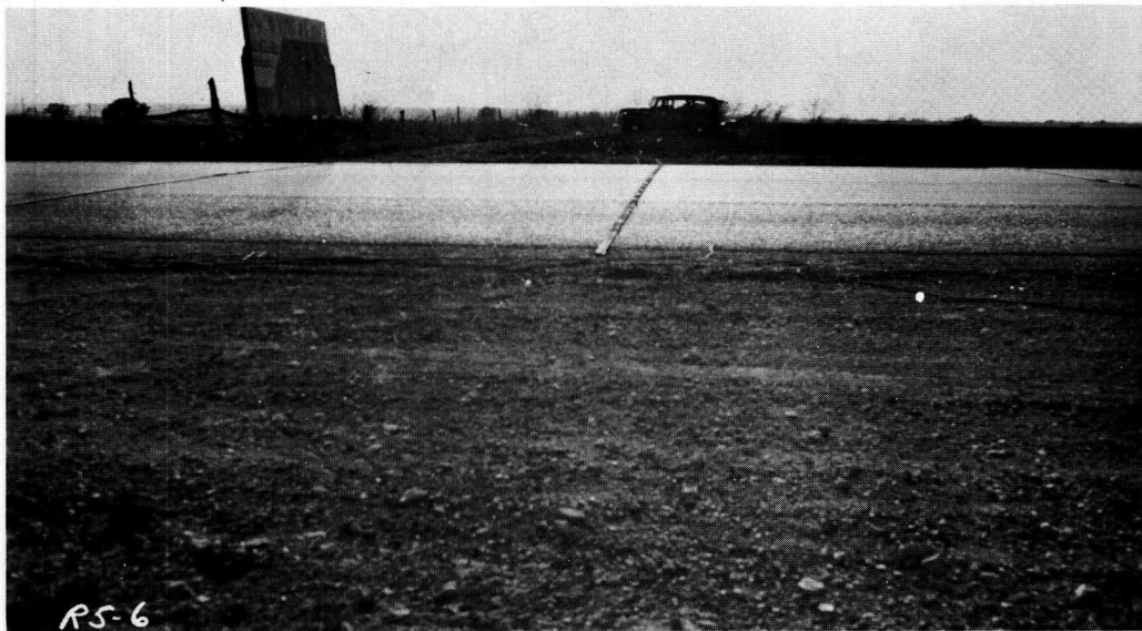
Figure 1. View of lateral placement and speed tapes with recording truck in the background.
