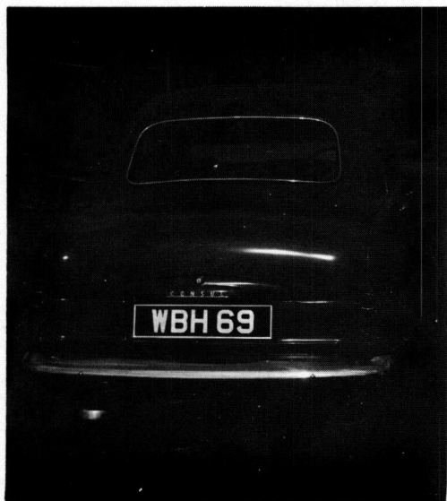
Figure 9. Rear view of a car with a moderate amount of chromium, taken in sunlight but printed so as to show several high lights. The distorted image of the sun at the right of the bumper has an intensity of the order of 5,000 candelas several hundred times greater than the adjacent flasher. The good background conditions higher on the vehicle will be noted.
