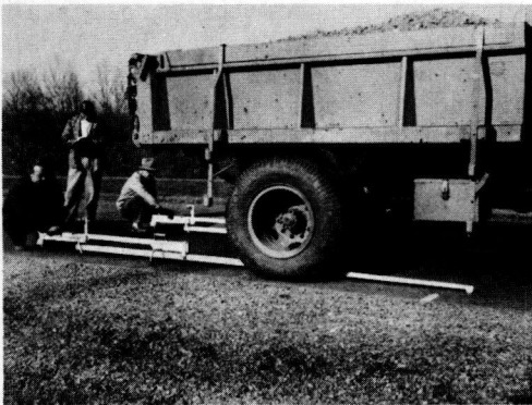
Figure 1. Deflection indicators in position at beginning of test.
