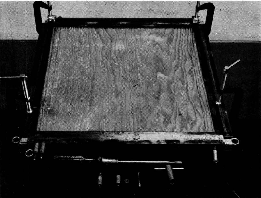
Figure 2. Combination tensioning frame and casting form used in constructing the test slabs. Anchorage device for maintaining wire tension is shown in the foreground.
