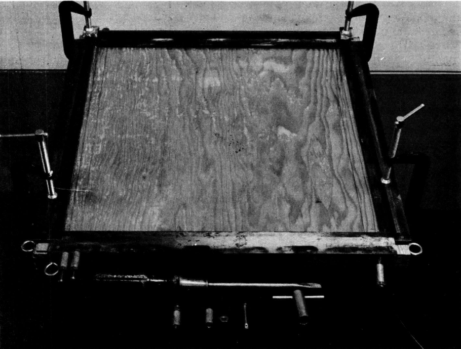
Figure 2. Combination tensioning frame and casting form used in constructing the test slabs. Anchorage device for maintaining wire tension is shown in the foreground.
