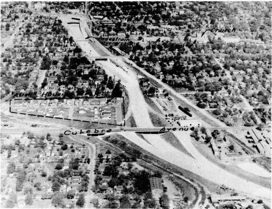
Figure 2. Route 87 After Improvement Showing Vehicle and Pedestrian Overpasses Provided to Link the Residential Area and the Left with the Community Center, Church, School, Etc., on the Right
