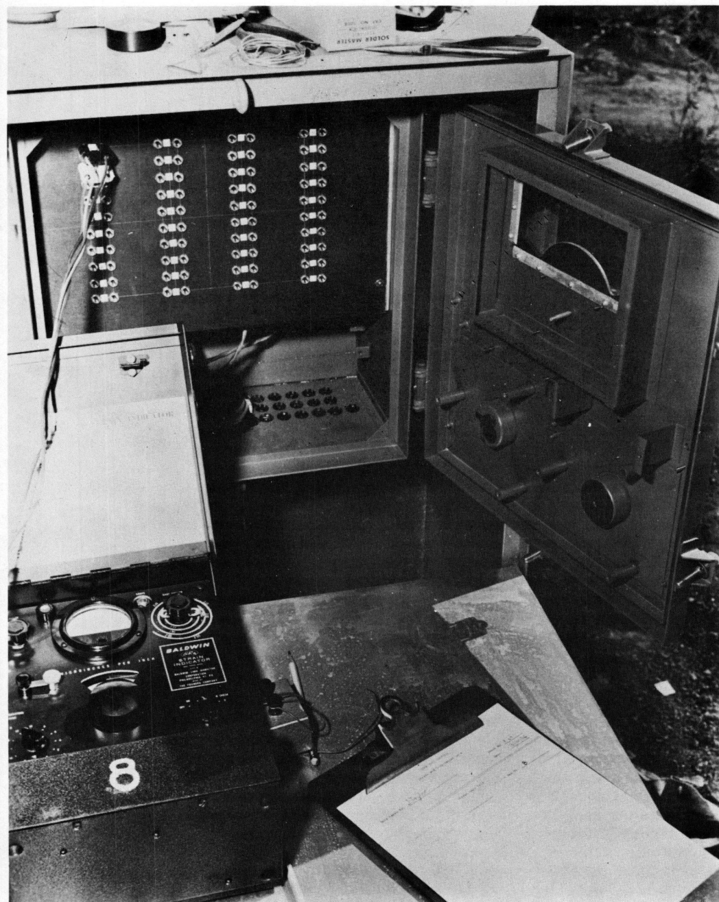
Figure 9. Terminal board ready for gage reading, showing indicator box and jack plugs inserted into board.
