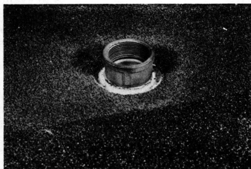
Figure 8. Machine faced pipe cap bonded to cored disc.
