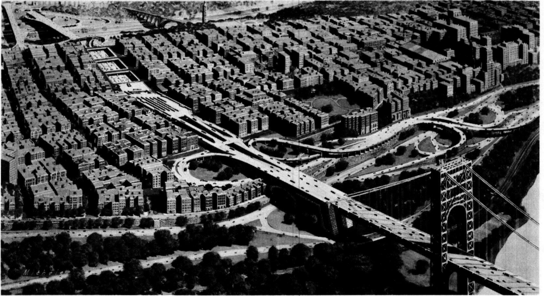
Figure 1. Artist's rendering of The Port of New York Authority's plans for improved Manhattan approaches to the proposed lower level of the George Washington Bridge showing new connections to Henry Hudson Parkway, the new Trans-Manhattan Expressway to connect with Cross-Bronx Expressway, and a suburban bus passenger facility.
