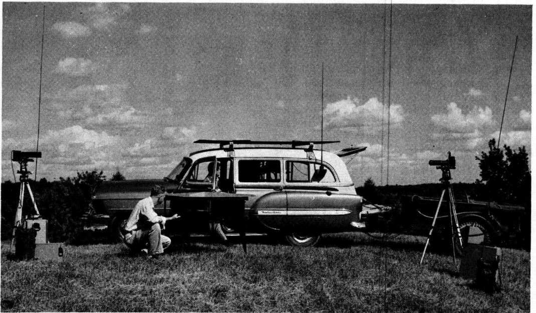
Figure 5. The amplifier controls and recorder for the Recording Polar Nephelometer, which is shown on the ground, are rack-mounted behind the front seat of the vehicle. When the two units of the Portable Transmissometer are used at long separation distances, radios (the antennae of which are visible in the picture) are used for communication.
