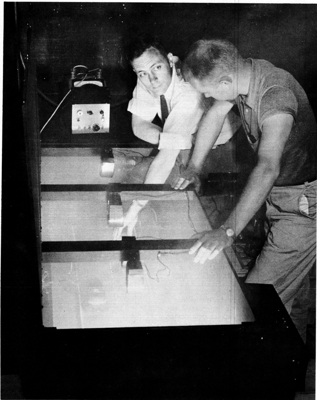
Figure 7. The covers of the "fog box" have been raised to attempt to show the 25:1 scale model cars immersed in artificial fog. The "peep hole" through which one obtains a driver's-eye view of the roadway is in the near end of the box.
