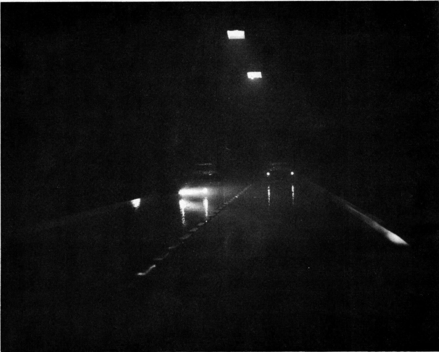
Figure 8. Improved highway lighting in fog. This photograph was taken through the peep hole in the fog box, with the taillights of increased candlepower on the receding car at the right, narrow beam street lights and "cross-eyed" low-mounted fog lights on the approaching car and the driver's car.
