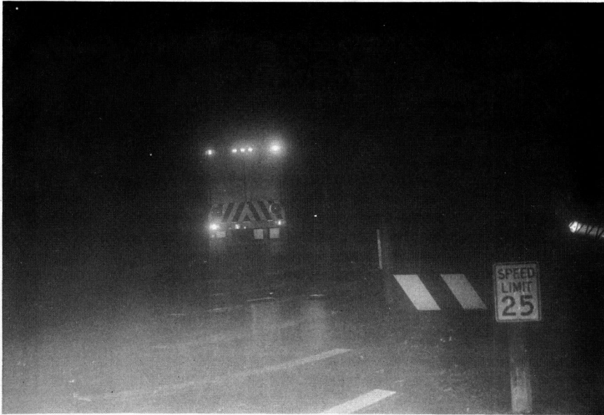
Figure 5. For vehicle-mounted lamps, a pair of PAR-36 clear fog lamps is mounted a few inches above the road surface. These were on in Figures 2, 3, and 4, but here are shown alone. This should be compared with Figure 6.
