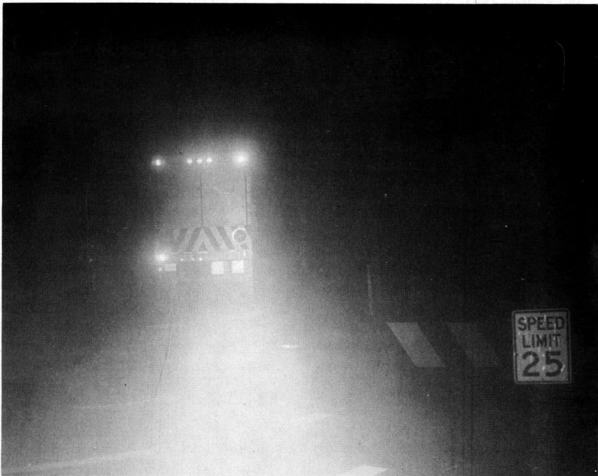
Figure 7. A 100-watt PAR-46 spot covered with a polarizing filter of about 40 percent transmittance is used alone here. This is equivalent to an unfiltered 40-watt except that the filter reduced the 140-deg back scatter (rainbow) which is strongly polarized.
