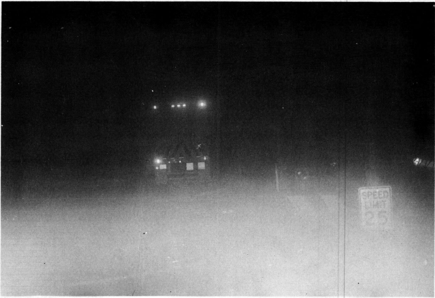
Figure 6. The lights used here, a pair of PAR-36 30-watt fog lamps, are the same as Figure 5 except that they have been raised to where the angles between light beams and camera axis correspond to those between head lamps and driver's line of sight in modern passenger cars.
