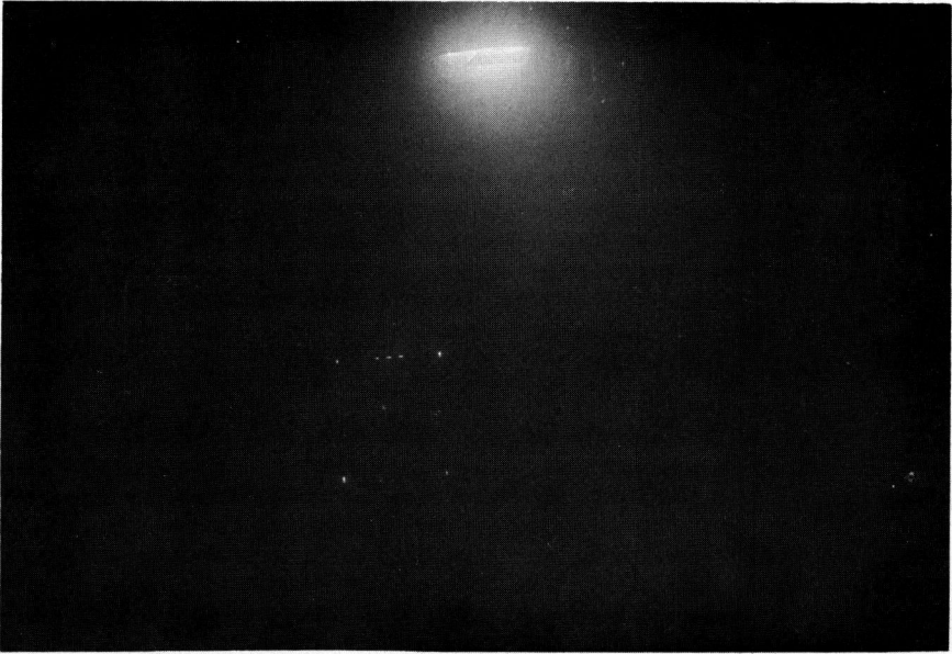
Figure 2. A luminaire of a type used in several toll roads is on in this picture. In this and the next two photographs the camera looks over a pair of low-mounted PAR-36 clear fog lamps. The common practice of showing lighted streets in the absence of headlamps seems unrealistic and increases the apparent value of silhouette seeing. The spotlight at the extreme right in this and several other pictures is part of the fog-regulating device.
