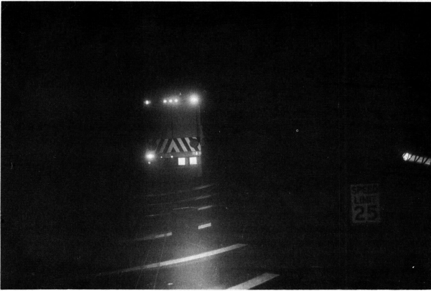
Figure 8. This differs from Figure 7 in that a crossed polarizing filter was before the lens. The exposure was increased to be sure of recording all low brightness areas. The back scatter from the beam is reduced to about 0.01 of that in Figure 7. The two squares at the lower right of the truck are retro-reflective sheets. On each side of the license are plastic prismatic reflectors.
