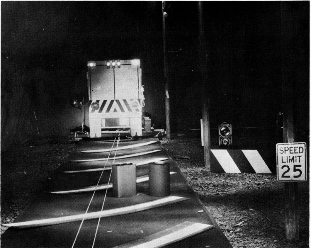
Figure 1. This is a fogless view of the scene shown in Figures 2 to 8. The road surface is 4 ft wide and 40 ft long, of rough textured hardboard sprayed with asphalt to simulate a black top road. The back of the truck is too large to this scale. It carries full size marker and turn indicators. The upper right and lower left markers are amber, the others red. The diagonal stripes are of beaded white paint scrubbed to give a traffic polished effect. The rectangular and cylindrical test objects in the foreground are painted dull black.
