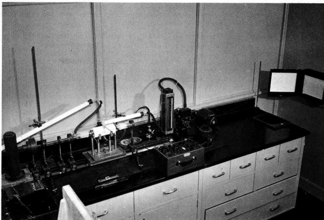
Figure 10. Stripping test equipment.
