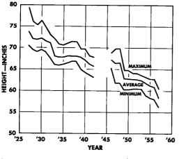
Figure 2. Car over-all height (car loaded).
