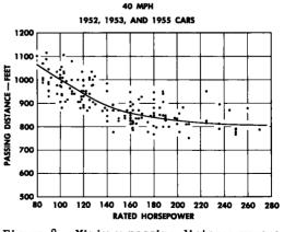
Figure 8. Minimum passing distance versus rated horsepower.
