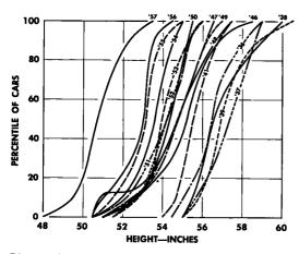
Figure 3. Driver's eye height to ground (defined according to visibility test procedure).
