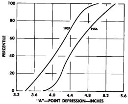
Figure 4. Front seat "A"—point depression percentile distribution.
