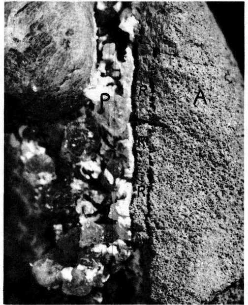
Figure 16. Another example of rim differentiation after mild acid leaching. Note that in this case a more soluble zone occurs on the inner side of the rim. A, unaffected aggregate; R, rim; P, cement paste.
