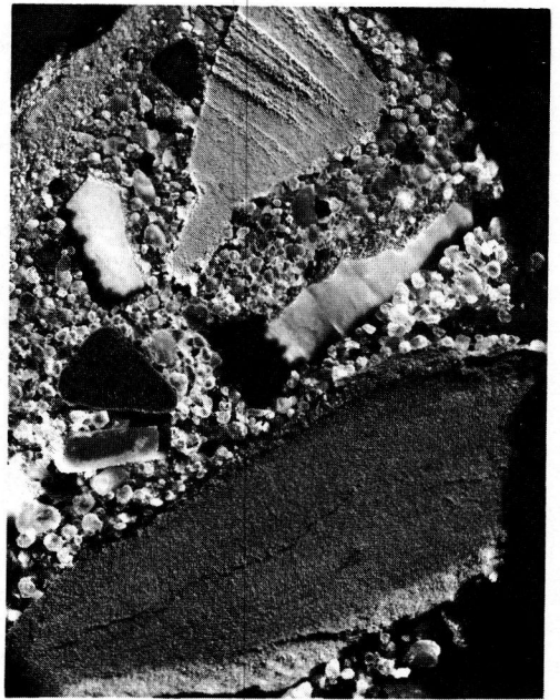
Figure 10. Acid etching readily attacks the pure limestones (B 1 and B 2 in Figure 9). Note that the aggregate-cement paste boundary of these particles is sharp.
